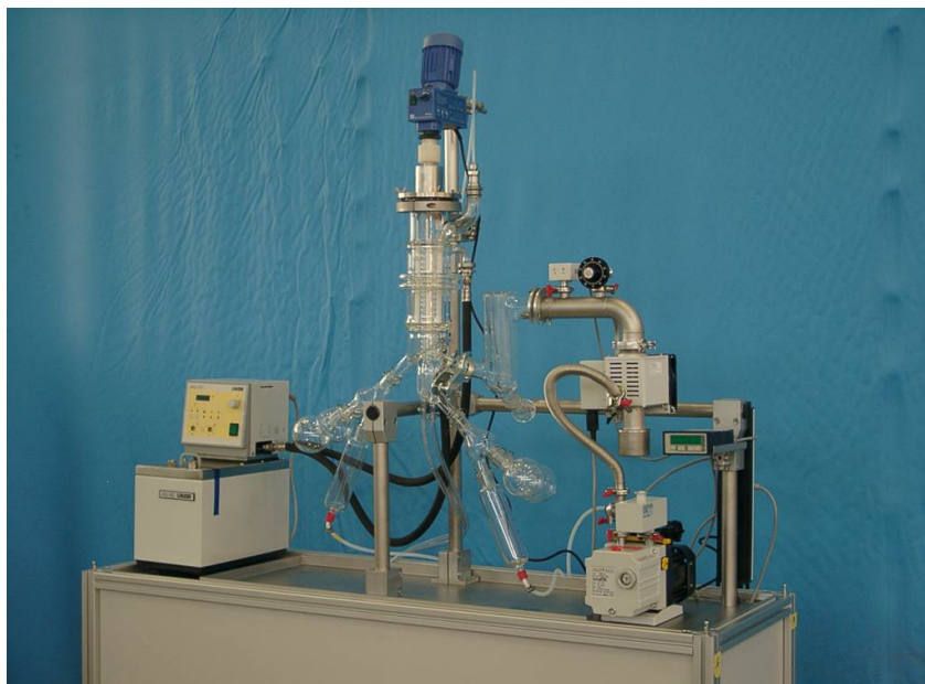
The Short Path Distillation Plant was designed by InCon's scientists to use in our own R&D lab.
